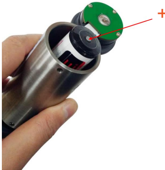
Figure 13. Facing the positive terminal up
