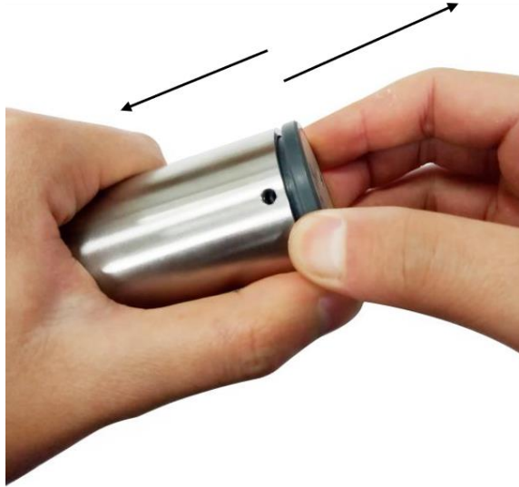
Figure 12. Pull open the battery cover plate slowly
