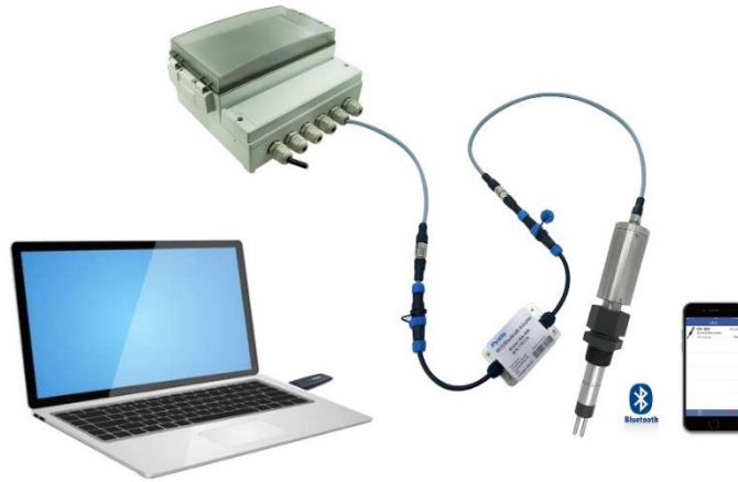
Figure 26. Connect to CR-300 via the Bluetooth USB adapter plugged onto the PC and the Bluetooth/WiFi adapter inserted between CR-300 and a controller as the power source
