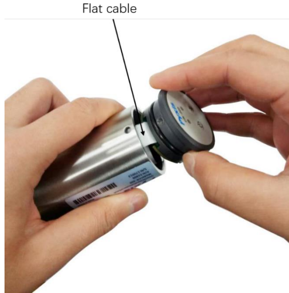
Figure 14. Place the battery cover plate back to CR-200
