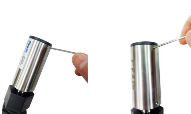
Figure 11. Loosen the battery cover screws
